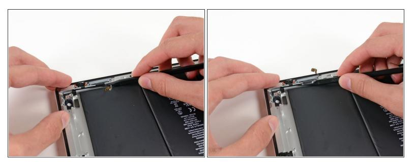
Using the tip of a spudger, release the adhesive underneath the volume button branch of the ribbon cable.
