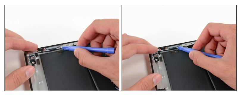
Continue sliding the plastic opening tool underneath the power & volume cables, releasing the adhesive.
