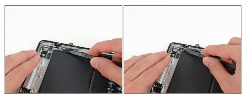
• Continue sliding the tip of the spudger toward the top of the iPad, releasing the adhesive.
