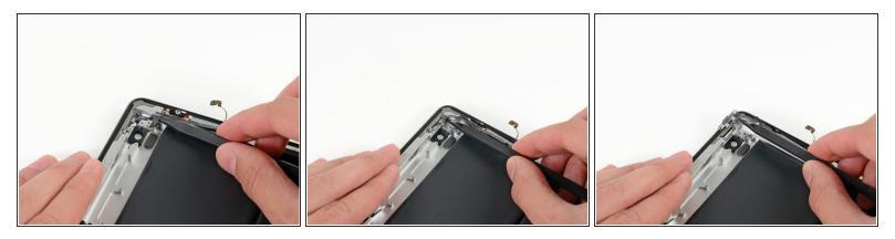
• With the tip of the spudger still underneath the ribbon cable, gently lift the power button out of its socket in the aluminum frame.
