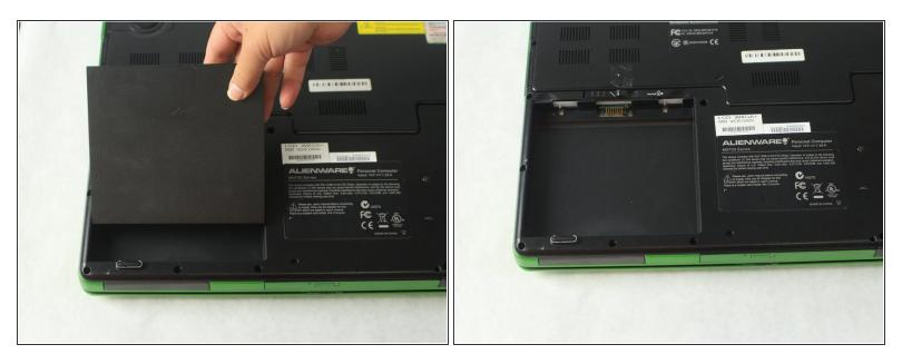
Now that the battery is free, use your finger to pry the battery upward, out of its designated compartment.
