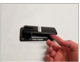
Place phone face-down and use your nail to pry the back off the back.
