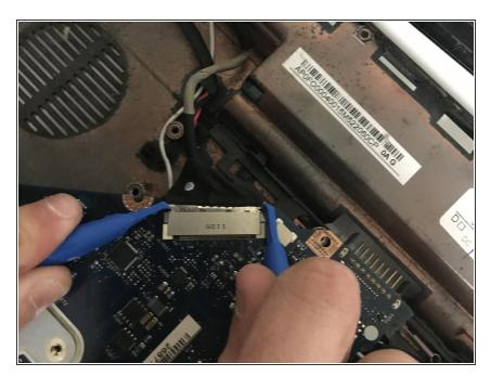
Remove the ribbon wire that connects the display to the motherboard using two plastic opening tools.
