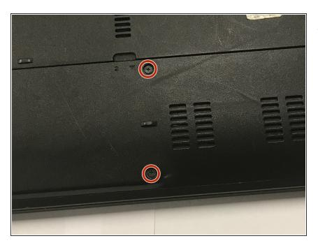
Remove the two 6.0mm Phillips #00 screws from the back cover.
