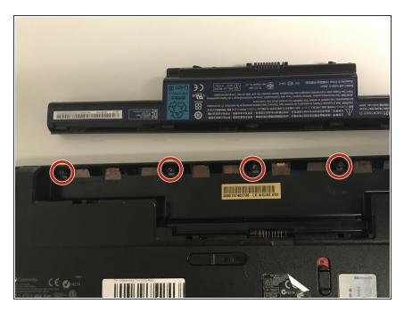
Remove the four 3.0mm Phillips #0 screws from the battery compartment.
