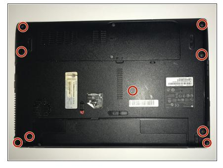
Remove the nine 6.0mm #00 Phillips screws from the back of the laptop.
