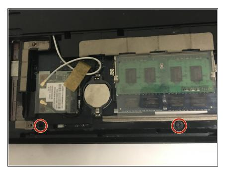
Remove the two 6.0mm #00 Phillips screws from the area under the back cover.
