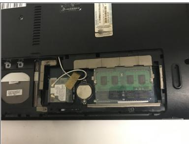
Remove the back cover by placing a plastic opening tool in the indention and prying upwards.
