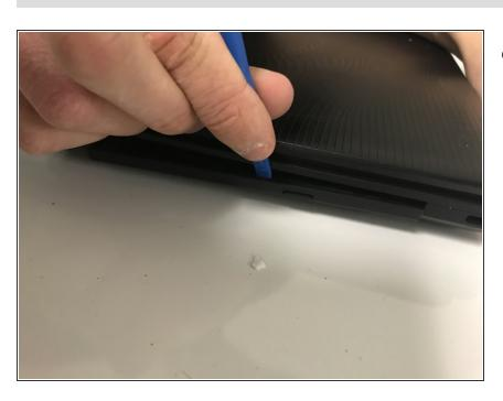
Use a plastic opening tool to remove the disk drive cover on the right side of the laptop.
