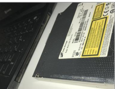
Use the metal spudger to pry upwards on the disk drive until you can grab and remove it.
