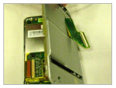
• Slide the circuit board through the slot in the keyboard.
