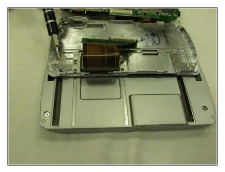
Remove the keyboard by unscrewing the two pairs of silver Torx head screws that run along the sliding tracks.
