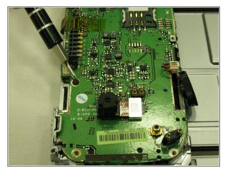
Secure the motherboard by screwing the small black Phillips head screw into place, located below the right speaker. Note: You may need to remove the right speaker in order to replace this screw.
