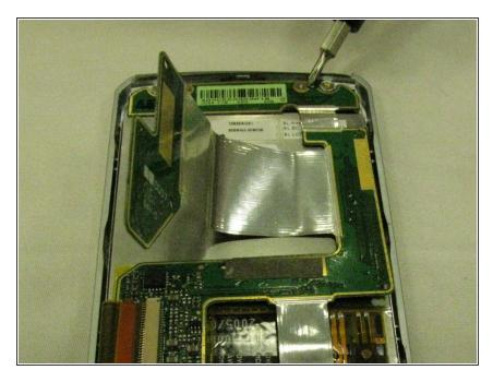
• Unscrew the four Phillips head screws that attach the screen to the front case.
