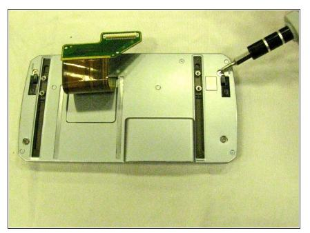
Remove the four silver Phillips head screws from the screened half of the phone.
