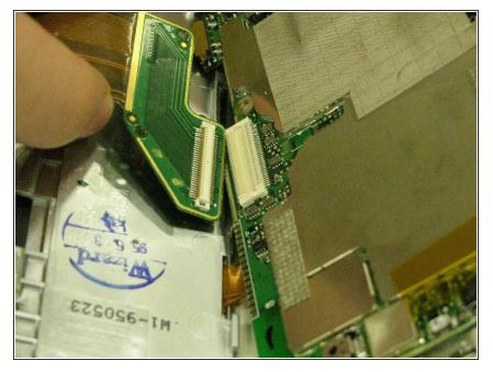
Attach the motherboard to the circuit board, aligning the two white rectangles until they snap into place. Lay motherboard into place.
