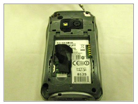
• Secure the back cover by screwing the four long, black Torx screws into the four corners of the back cover.
