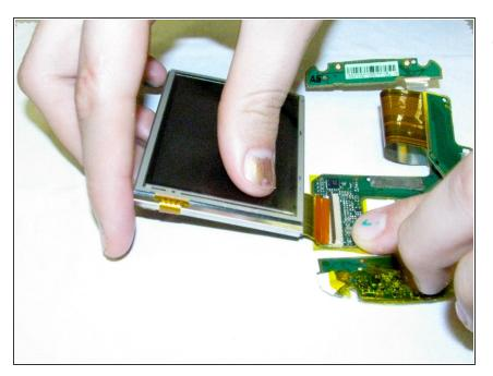
Attach the new screen by aligning the orange tab with the beige rectangle on the circuit. Secure by pushing down on the bronze piece.
