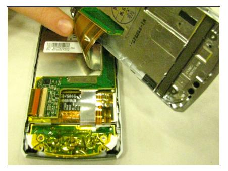
Use the light blue wedge tool to remove the back. The circuit board will slide out of the slot and will stay attached to the remaining front half of the phone.
