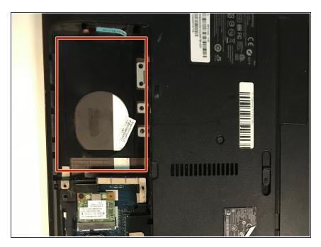
Remove the hard drive by lifting it out, and removing any necessary screws.
