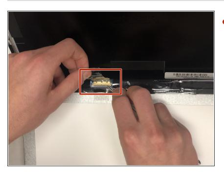
Pull the gold ribbon cable to disconnect the screen from the laptop.
