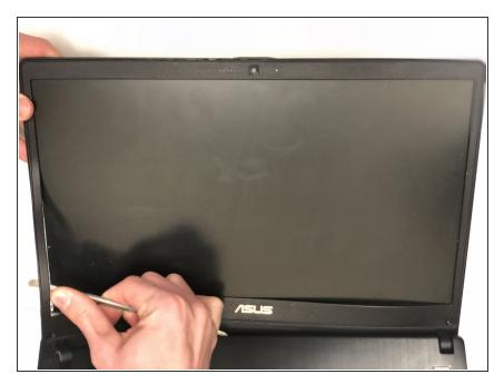
Pry the front edges of the screen using the spudger.
