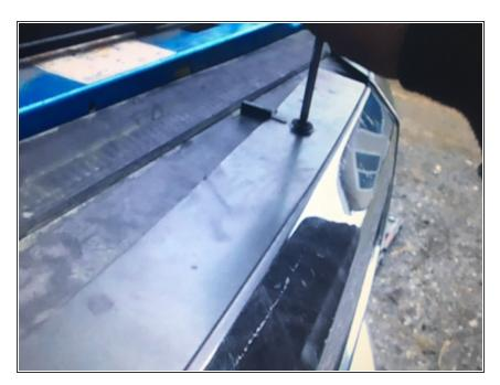
Remove the 5 screws with the screwdriver to remove the grill.
