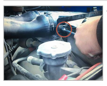
Set aside the windshield fluid/coolant reservoir by removing the 11mm bolt.
