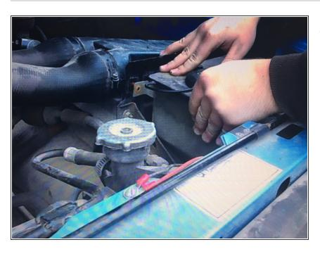
Reinstall the windshield fluid/coolant reservoir with the 11mm bolt.
