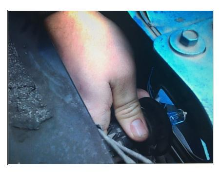
Reinstall the headlight bulbs by turning clockwise on the retaining clip.
