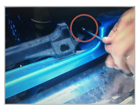
Remove the bolts retaining the header panel using the 8mm socket and ratchet.
