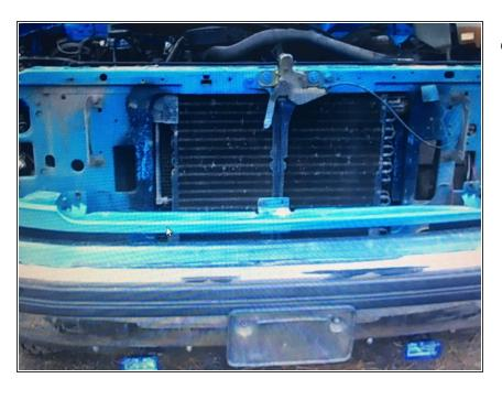
Remove the old header panel, and install the replacement panel.
