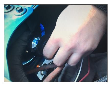
Remove the headlight bulbs from the headlight housing by turning them counterclockwise on the retaining clip.
