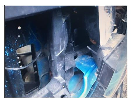
Reinstall the headlight bezels after reinserting the marker lights with the two screws, and two 11mm bolts.
