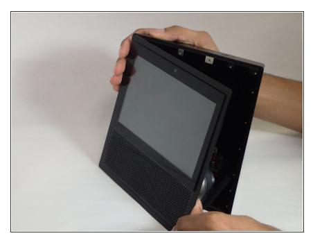
After the screws are removed, grip the front panel and remove, using a plastic opening tool if necessary.
