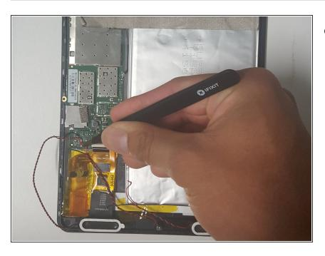
Remove the wires with the tweezers by pulling them upward.
