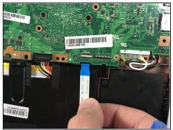
Use the plastic opening tool to flip up the small clamp and pull out the ribbon cable.
