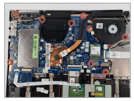
Use a PH00 screwdriver to remove the nine 3mm screws.
