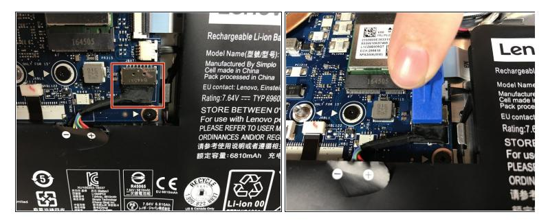
• Use your fingers or an opening tool to slide the battery connector out of its motherboard socket.
