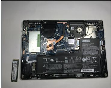
• Use your fingers to lift up the SSD and pull away from the socket removing it from the laptop.
