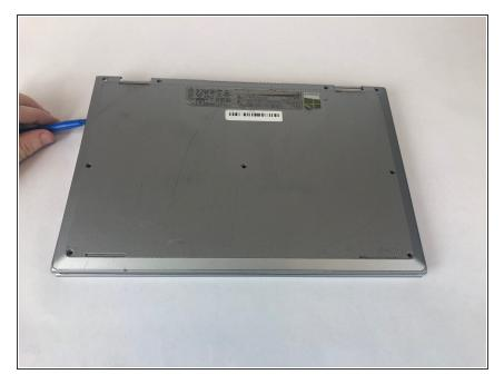
Use a plastic opening tool to remove the cover from the back of the computer.
