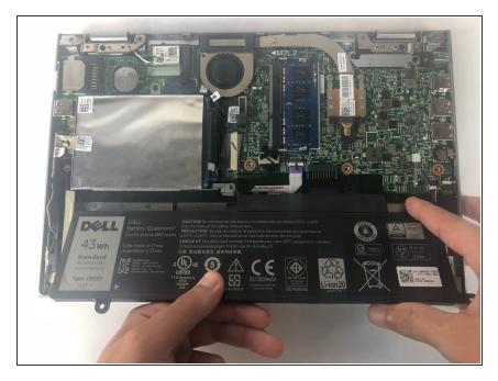
• Lift the battery up and toward yourself to remove it, revealing the back of the keyboard underneath.
