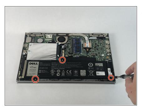
• Remove the three small 4.7mm PH0 screws that secure the battery.
