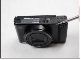
• Use the plastic opening tools included in the iFixit tool kit first. If the shell/parts do not detach from each other, use metal spudgers as a last resort to loosen/separate the plastic shell of the camera. Keep in mind that there may be more screws holding parts together. Work delicately and separate sides evenly.
