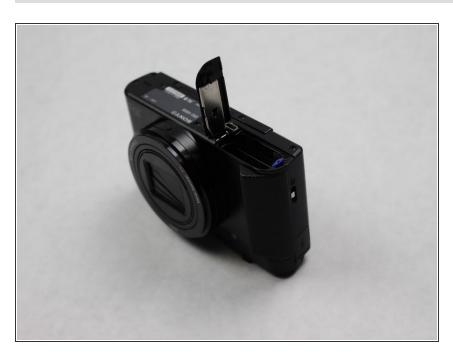
Open the compartment located at the bottom of the camera. Slide the LOCK/OPEN switch to the OPEN side. Locate the small blue tab on the side. Pull it in direction away from battery. Remove the battery and set it aside.
