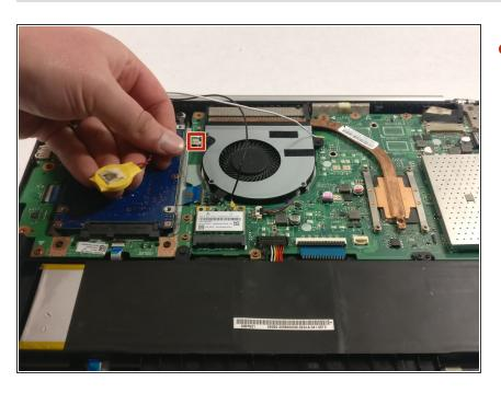
Disconnect the CMOS battery and its wire from the connector. The CMOS battery is now disconnected from your device.
