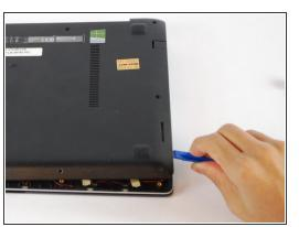
• Use a plastic opening tool to gently pry the bottom of the laptop up. Slowly slide it along the edges, twisting it every so often to pop the bottom of the laptop out of the clips holding it in place.
