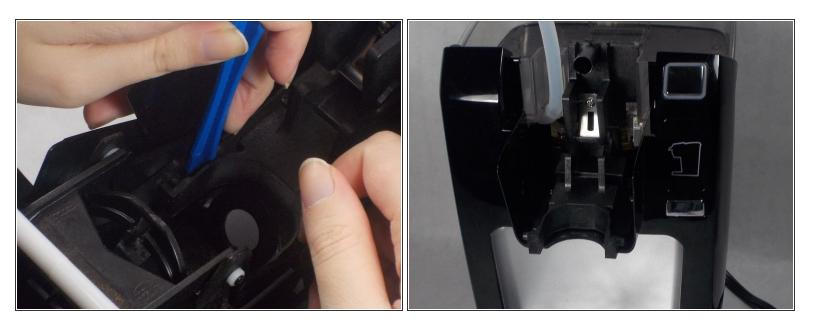
Using the iFixit Opening Tool, gently pry apart the plastic head assembly piece from both the body's axles and its left to remove it.
