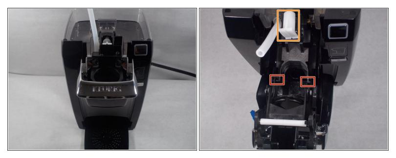
Pull the head assembly forward to reveal the two plastic axle points that keep the head assembly attached to the base.
