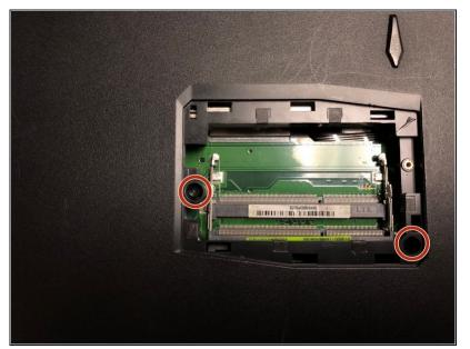
• Remove the two screws from underneath the RAM cover.
