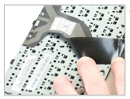
Check for visible damage on the ribbon cable such as folds, kinks, or corrosion.
