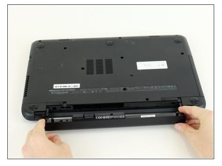
• Pull on the battery to remove.
