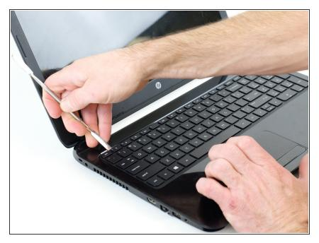
Using either a credit card or flat spudger, wedge it between the palm rest and the keyboard.
