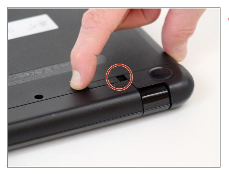
Slide the latch towards the center of the laptop so the unlock emblem appears.
