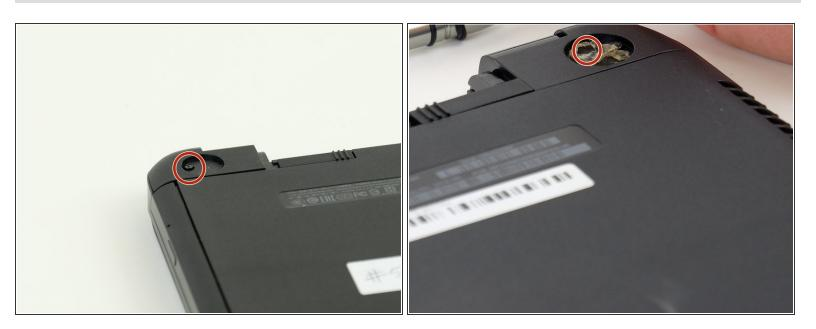
Now remove the two Phillips screws that are located below the rubber feet.
