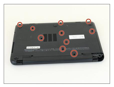
Using the Phillips #00 screwdriver, remove the 5 millimeter screws that are visible.
