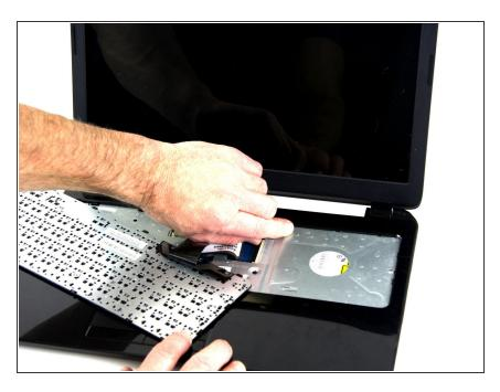
Remove the ZIF connector that connects the laptop to the keyboard cable.
