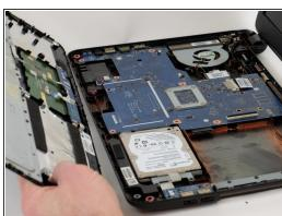
Carefully remove the palm rest and flip it over.
