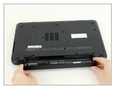
Pull on the battery to remove.
