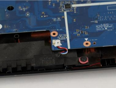
• Lift up on the speaker connectors to unplug the speaker cables.
