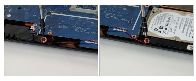
Remove the screws that are securing the speakers.
