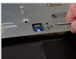
Disconnect the touch pad ribbon cable by lifting up on the connector.
