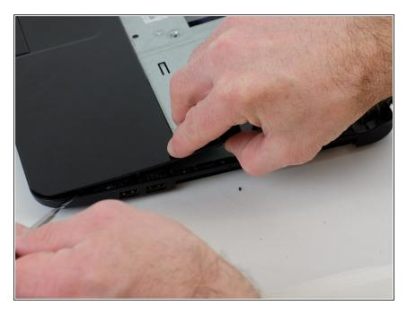
Work the spudger in small increments around the palm rest while lifting it up in the air.
