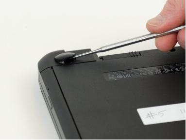
Using the spudger, remove the two rubber feet that are located near the battery.
