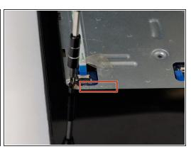
Now remove the screws indicated by an arrow stamped into the metal, located where the keyboard was.
