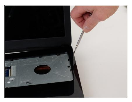
Take the metal spudger and gently insert in between the palm rest and the body.
