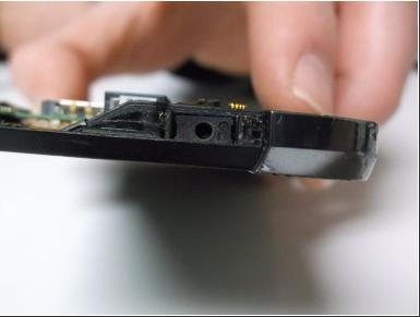
Remove the power button with the tweezers.
