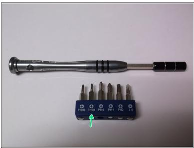
Use a PH00 screwdriver to remove the 6 screws from the mid-frame.
