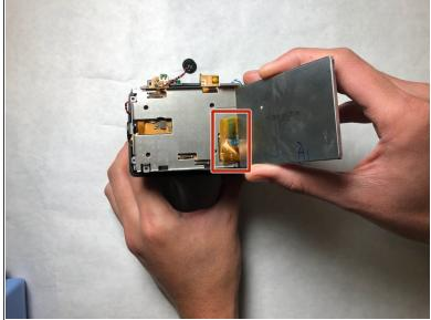
Carefully remove the LCD screen.
