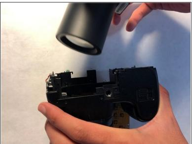
Remove the inner lens.
