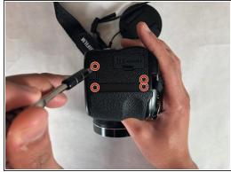
Using a Phillips #000 screwdriver, remove all of the 4mm screws from the left, right, and bottom of the camera.
