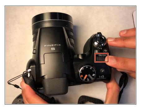
Turn off the camera by pushing the ON/OFF switch as shown.
