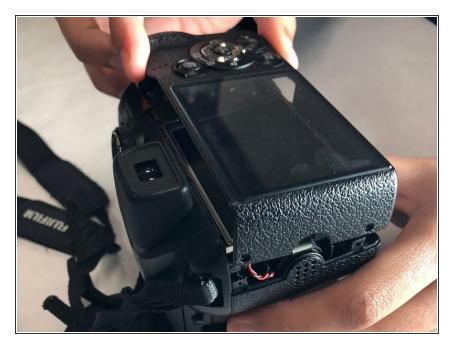
Remove casing part pictured by gently pulling up until casing is fully detached.
