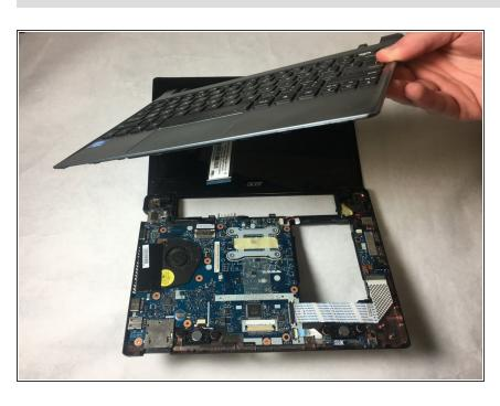
Lift the keyboard off of the back casing.
