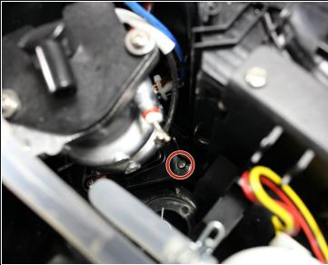
Using a #1 Phillips head screwdriver with an extension, remove three 6mm screws holding the heater to the unit.
