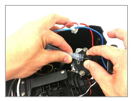
Detach the valve tubes from the device by pinching the pins and sliding the valve tubes off.
