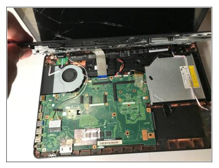
• Separate the keyboard from the computer to expose the inside of the computer.
