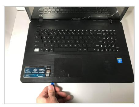
Once the screws are out, open up the laptop and use the plastic opening tool on the keyboard and the back to pry it open.
