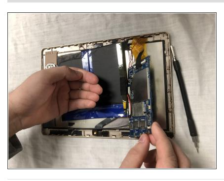
Once screws are removed, carefully remove the motherboard out of encasing.
