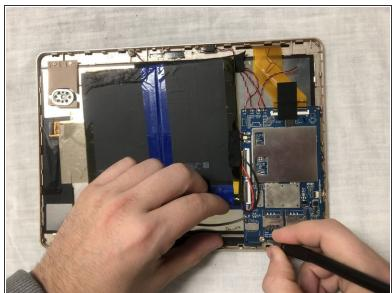
Use flathead screwdriver tool to remove the three 2.5 mm screws shown in the photo. Two screws are located at the base of the motherboard and there is one screw located at the top.
