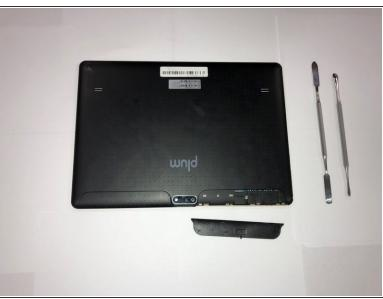
Use a metal spudger to remove the small panels to the immediate left and right side of the camera.
