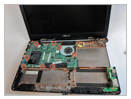
Remove the eight 5.7mm screws using the Phillips #0 Screwdriver.
