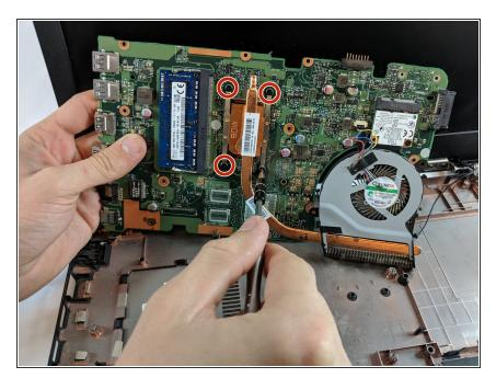
Unscrew and remove the four 0.01mm screws using the Phillips #0 Screwdriver from the heatsink.
