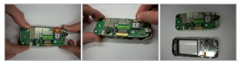
• On the rear phone casing, locate the ribbon cable tab and connector next to the SIM card port.
