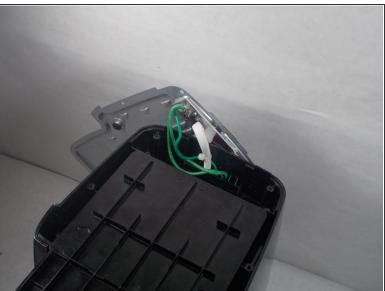
Reposition the metal lid while keeping the heat sink attached in order to reach the screws underneath.
