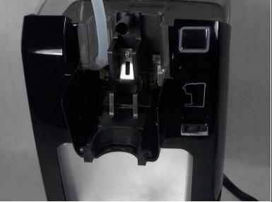
Using the iFixit Opening Tool, gently pry apart the plastic head assembly piece from both the body's axles and its left to remove it.
