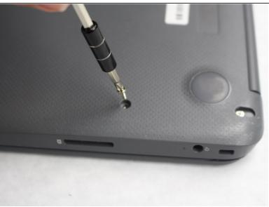
Position your closed laptop face down to remove the 9 visible 6mm screws using the Phillips #1 screwdriver.
