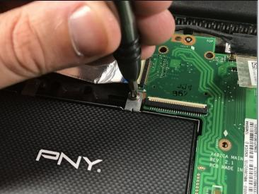
• Remove the four 5mm screws that attach the hard drive bracket using the Phillips #0 screwdriver.
