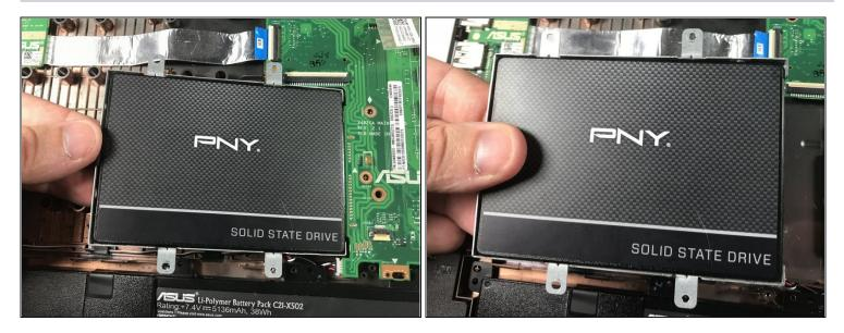
Lift the hard drive and attached bracket up and out.
