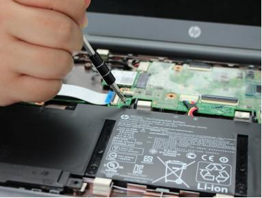
Remove the six 4 mm screws holding the battery in place with a Phillips #1 screwdriver.
