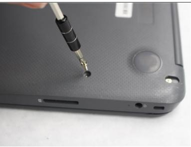
Position your closed laptop face down to remove the 9 visible 6 mm screws using a Phillips #1 screwdriver.
