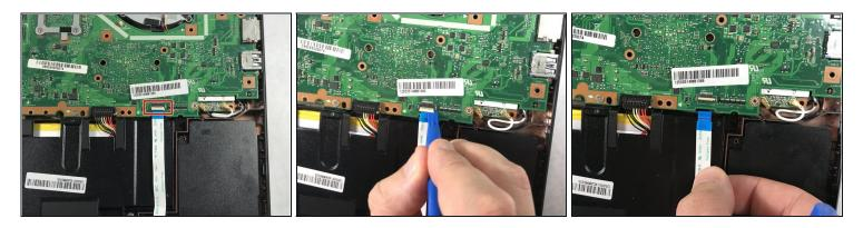
• Use the plastic opening tool to flip up the small clamp and pull out the ribbon cable.
