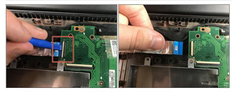
• Unplug the power strip connecting to the motherboard with your fingers or plastic opening tool.
