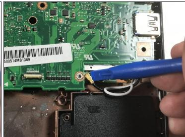
• Use the plastic opening tool to unclip the two wires from the Wi-Fi card that are connected to the motherboard.
