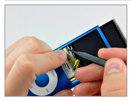
While holding the light colored socket down with one finger, use the tip of a spudger to flip the ZIF cable lock up toward the bottom of the Nano.
