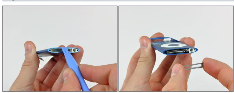
Use an iPod opening tool to pry the aluminum dock bezel out of the Nano.
