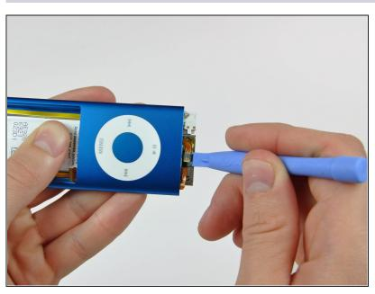
Use the edge of an iPod opening tool to peel the click wheel ribbon cable and its ZIF socket off the dock connector.
