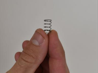
Remove the unwanted spring and place your new spring back into the hole.
