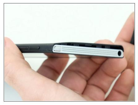
Gently pry up on the plate with the spudger. You may hear some cracking noises as you work the spudger around your device, this is normal.
