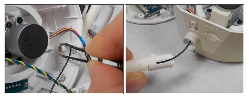
Pinch the WiFi antenna's clip mount inside the upper part of the body with blunt ended tweezers while pulling the antenna from the outside. To reassemble your device, follow these instructions in reverse order.
