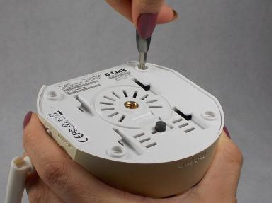
Using a #1 Phillips screwdriver, remove the four 7mm screws that are exposed by the removed feet.
