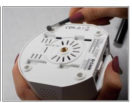
Locate and remove the four rubber feet on the bottom of the camera using your fingers or a pair of tweezers.
