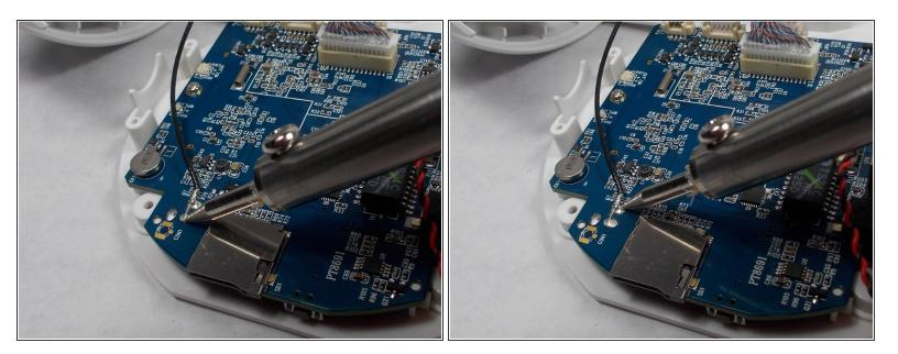
Using your soldering iron, heat the antenna contacts on the motherboard until the wire releases.
