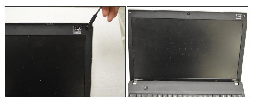
Then, use the end of a spudger to remove the two screw covers from the top and bottom corners of the display.
