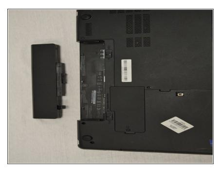
Remove the battery from the device.
