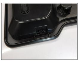
Bend each metal flap straight up with the pliers to allow the metal cover to slide off.
