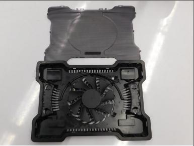
Remove the cover and expose the inside of the Cooler.
