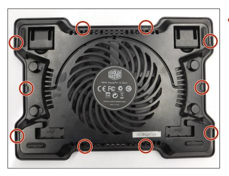
Flip the Device over and find ten folded metal slots holding the metal cover onto the base.
