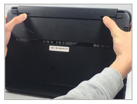
Press the two buttons inward to unlock the battery.
