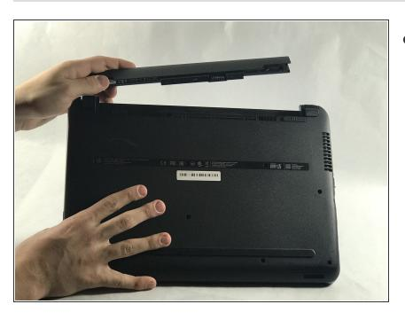
Remove the battery by pulling it from the slot.
