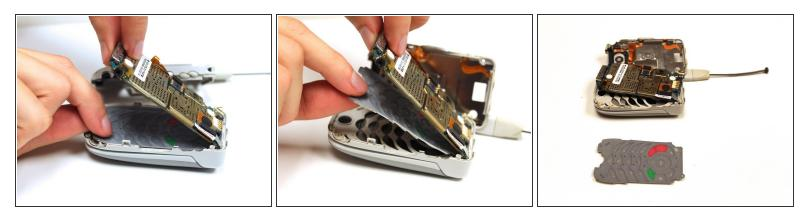
• Gently lift the end of the circuit board farthest from the phone hinge.
