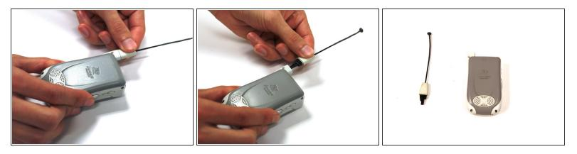
• Remove the antenna by grasping from the white plastic piece just below the antenna and pulling away from the phone.
