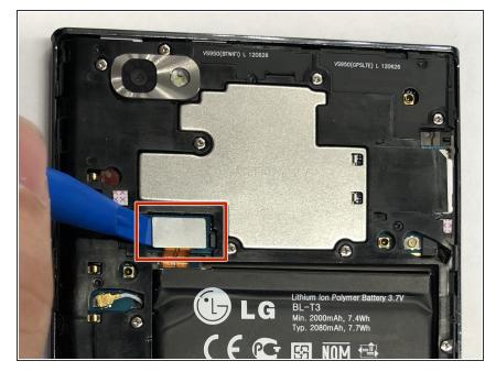
Carefully use the plastic opening tool to pry the ribbon cable connecting the battery to the motherboard of the phone.
