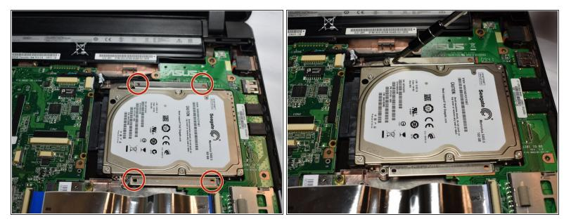
Using a Phillips #0 screwdriver, remove the four 4mm screws connecting the hard drive.
