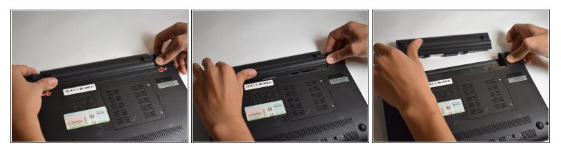
• Slide the tabs outward to remove the battery.
