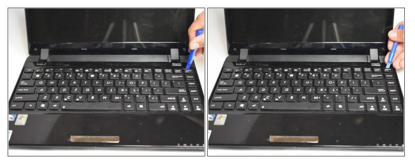
• Use a plastic opening tool and carefully pry the top panel from the base.
