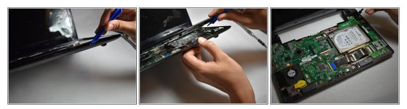
• Using a plastic opening tool, remove the top panel of the laptop.
