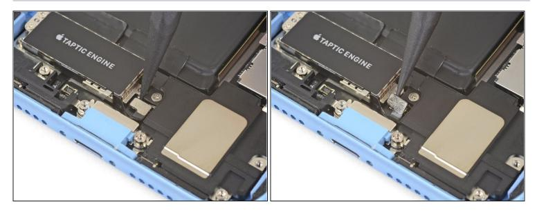
• Use a spudger to disconnect the Taptic Engine flex cable by prying it straight up from its socket.
