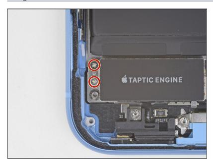
• Remove the two 1.8 mm Phillips screw securing the Taptic Engine.
