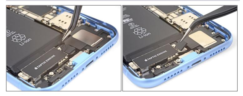
• Remove the piece of black tape and the small rubber rectangle covering the Taptic Engine connector cover.
