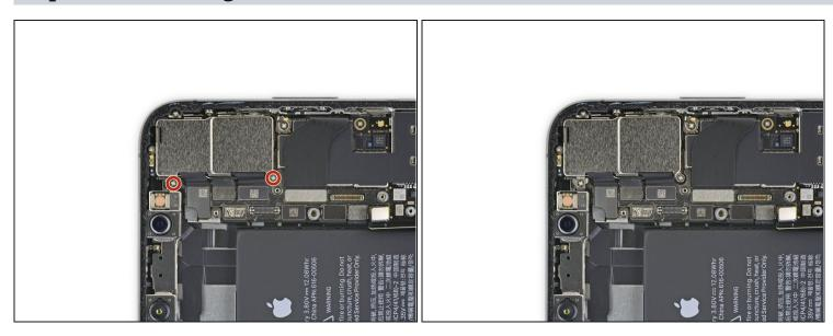
• Remove the two 1.8 mm Phillips screws securing the rear camera cover.
