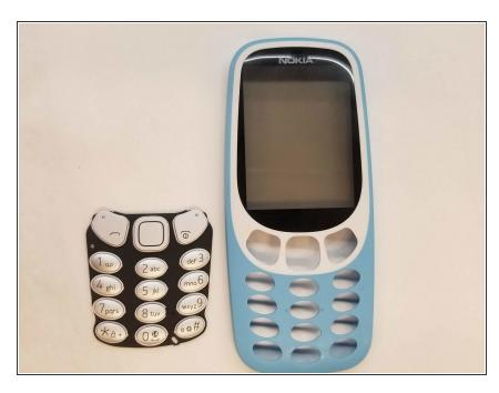
Using your finger, push the keyboard insert out of the front outer frame.
