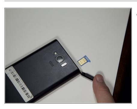
Make sure SIM card is debris free and placed properly on the tray.
