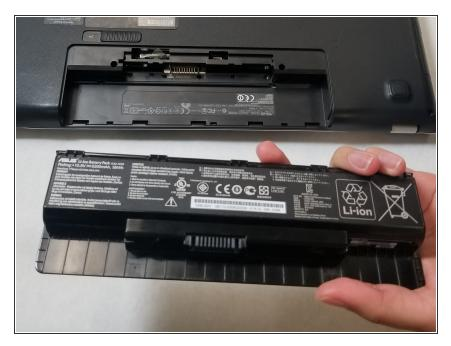
Keep the battery latch held while you remove the battery.
