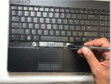
• Remove the six 3.63 mm JIS #0 screws holding the keyboard in place.
