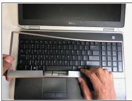
Pry off the plastic keyboard trim. It is easiest to start at the bottom of the keyboard.
