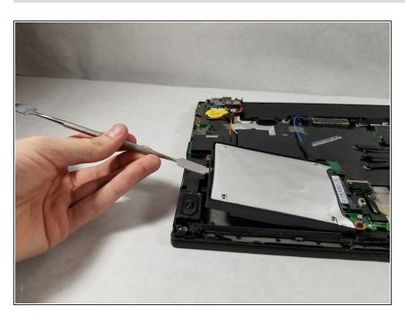
Use the metal spudger to lift the hard drive out of it's compartment.
