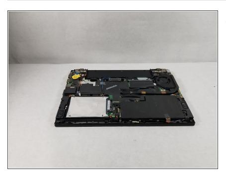
Remove the back panel from the device.
