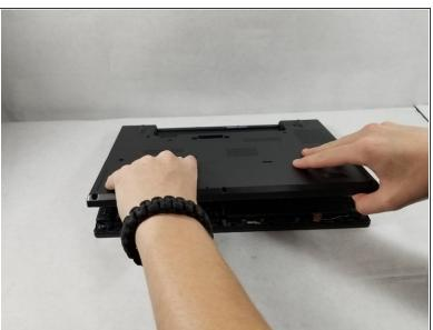
Using the metal spudger, wedge it in the seam where the backplate meets the front plate and run
