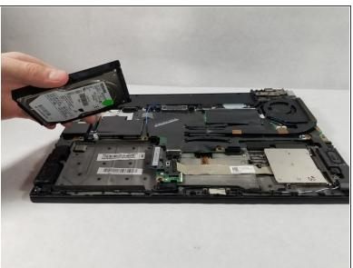
• Grab a hold of the hard drive and pull it straight out from the device.
