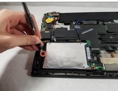
• Use the Phillips #1 screwdriver to remove the single screw securing the hard drive.
