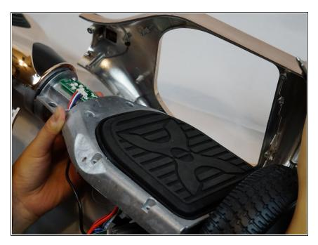
Separate the upper shell from the metal layer inside.
